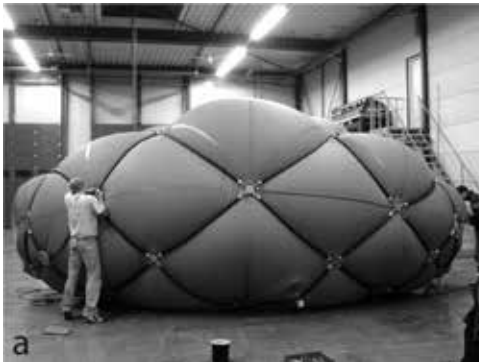
III. 17. Installation showing the action of pneumatic muscles: a) skeleton composed of pneumatic muscles, b) the whole structure is composed of pneumatic muscles and a shell.
