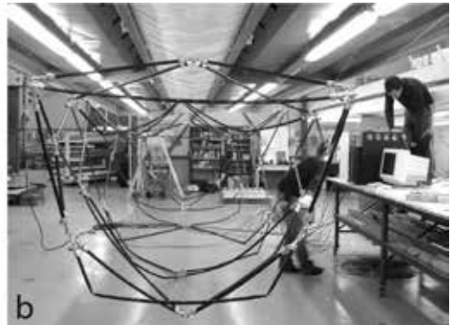
III. 17. Installation showing the action of pneumatic muscles: a) skeleton composed of pneumatic muscles, b) the whole structure is composed of pneumatic muscles and a shell.
