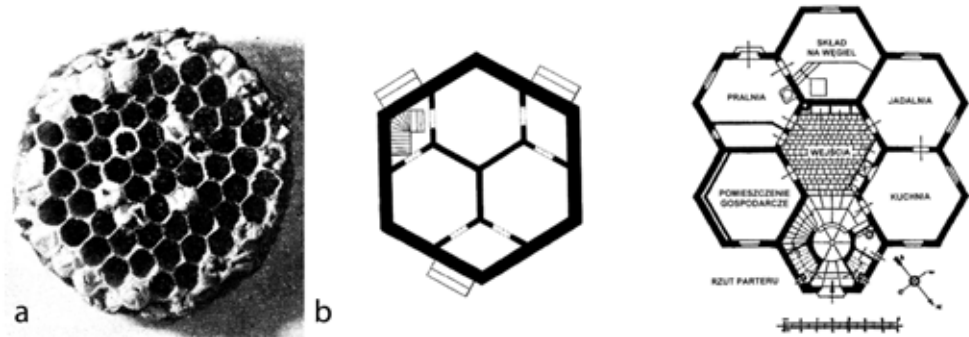
III. 13. Prefabrication in nature and construction: a) a hornet's nest, b) an example of using the insect's nest shape in construction is the hexagonal dwelling house from 1869 designed by Harriet Morrison Irvin and another around the year 1927 by Wilhelm Ulrich.
