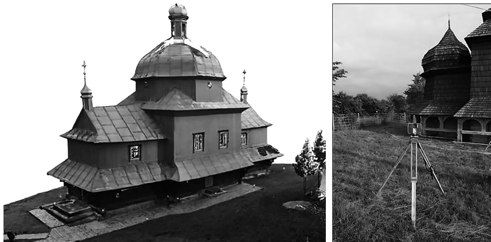
Ill. 7. Digital model of the wooden church Pr. Mother of God in the village Velikopole of Yavoriv district. Church scanning process, source: 3D scan of the wooden churches of Lviv region, op. cit.
