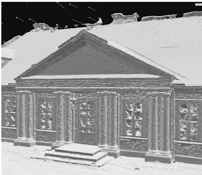
Ill. 4. Mesh model generated from drone photographs, 2025, source: work of Alicja Pijewska
