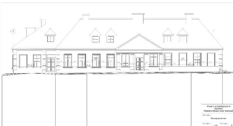
III. 6. Generated inventory from model in Revit, 2025, source: work of Julia Gonet
